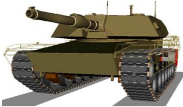
Figure 1: Multibody model of M1A1 Abrams tank in Universal Mechanism software, 371 bodies, 1916 d.o.f.
